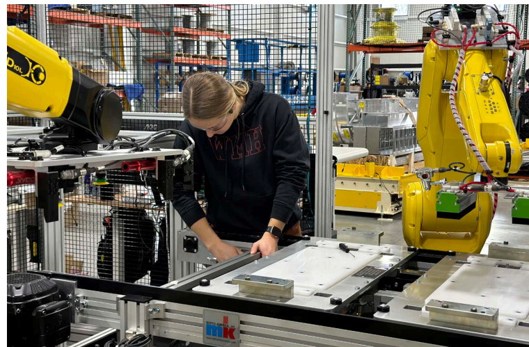
Mission Machine Build Assistant, Sophia DeGraff, assembling an industrial conveyor for an automotive customer.
